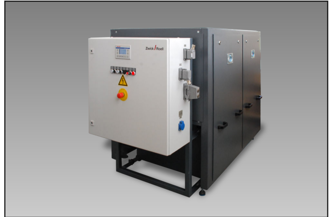
20-liter hydraulic power-pack with acoustic hood
